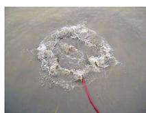
The bubble-mass drags the contents of the basin in its vertical wake. When the bubble mass hits the surface, the mud is re-suspended in the water, ready to be pumped out.
