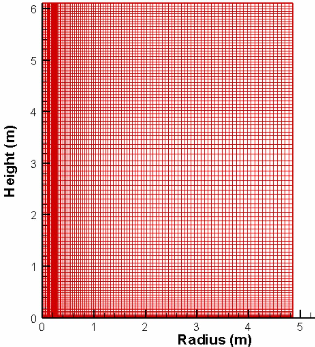
**Figure 3. The CFD Model and mesh for a large bubble rising in a cylindrical tank.**
