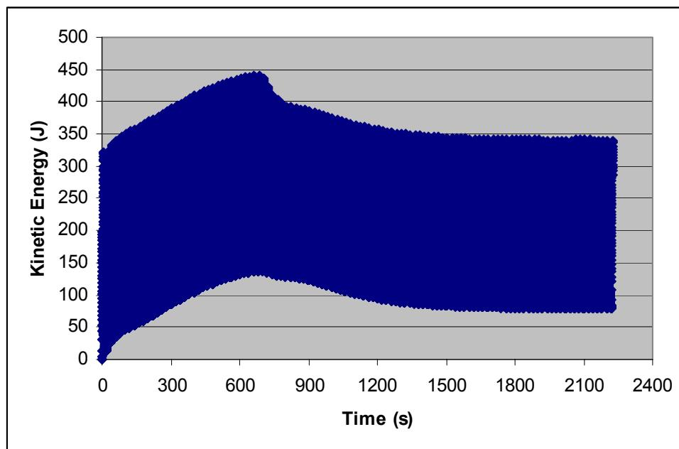
**Figure 8.** The Kinetic Energy in the tank as a function of time with a virtual wall.
