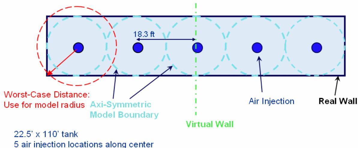
Figure 2. Pictorial of a 22.5' x 110' tank with 5 PHi forming plates installed.
