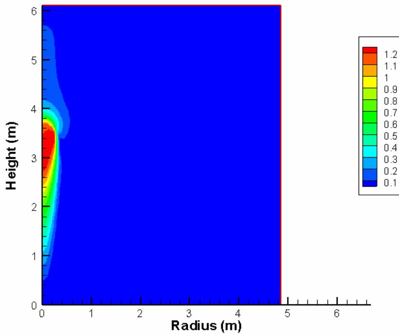
**Figure 4.** Velocity plot (m/s) of the model with real wall at  $r = 4.85$  m at  $t \approx 15$  minutes.
