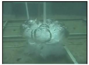
of odors because of the top grease layer going septic, then the mixer will have moved this material to the pumps, and the odors would be removed as well. If the odor is being generated from an up stream source, then the mixing would have no effect in removing odors. If an additive is being applied, then it will be more effective as it will be mixed well into the sewage.
